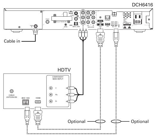
Note: Only (1) HDTV video connection needs to be made to an HDTV.
